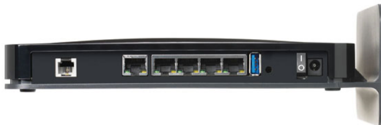
DSL line in, gigabit WAN port, 4x gigabit Ethernet ports, USB port, power switch and power jack. There's another USB port on the front — both are only USB 2.0, despite the blue colouring.
